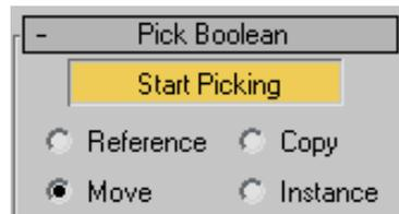
The subtraction Boolean operation subtracts the common area shared by the array box and the *Tower* object. You will later add a design element in the gap you just created.
