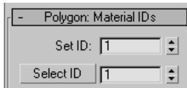
In its current state, if a material was assigned to any part of the *Tower* object, all its polygons would receive the same material. This is because they all have the same material ID number.
