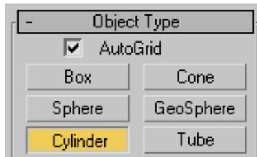
With AutoGrid on, you can create the object on top of an object you select in the scene.
